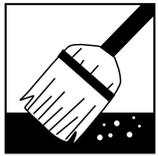
All backing surfaces must be structurally sound, level, true, dry, clean, and free of deleterious substances (wax, sealer, etc.), which may act as bond barriers (conforming to the industry standards as outlined by the TTMAC and the TCA). Ensure that all cracks and voids are cleaned and filled with a polymer modified thin-set mortar.
