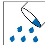
In a clean container, pour water and gradually add SILICAFLEX. Mix slowly to obtain a homogeneous and smooth consistency. Let sit for 10 minutes and mix again, but do not add water, latex additive or powder. During use, mix the mortar periodically, but do not add water.
