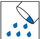
Pour 5.7 L of water into a clean container. Add 22.7 kg of NIVEX. Mix until an homogeneous, creamy (almost liquid), lump free paste is obtained.
