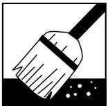
All backing surfaces must be structurally sound, dry, clean and free of dirt, oil, grease, paint, wax, curing agent or other deleterious substances, which may act as bond barriers. Surfaces that were previously in contact with one of these substances must be sanded, smoothed, stripped or scarified. They must also be treated with PX PRIMER. It is your responsibility to be sure
