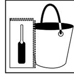
Use a rubber float and apply a firm pressure to completely fill the joints with grout. Remove excess grout on tiles also using a rubber float.
