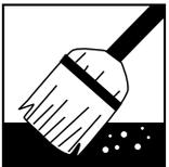
Before grouting, wait until the mortar or adhesive under the tiles is completely dry as per manufacturer's recommendations. Joints must be clean and free of dust. Make sure that at least 2/3 of the height of the joints is mortar free so that the grout can properly adhere within the joints.
