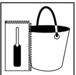
Pour the entire content on the surface to be levelled as soon as possible. In the corners of the rooms, spread with a squeegee or finishing trowel. As this is a self-levelling underlayment, no smoothing is required. It is recommended that you organize your work in such a way that the product can be applied in a continuous manner.
