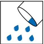
Pour 5.7 L of water into a clean container. Add 22.7 kg of FLEX 24. Mix until a homogeneous, creamy (almost liquid), lump free paste is obtained.
